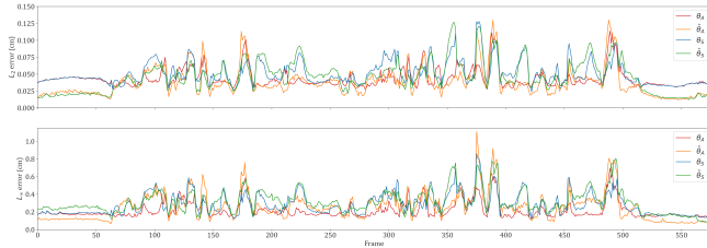
Fig. 9. A 573 frame pangram was used to test the tracker’s ability to invert the rig and match the reconstructed geometry. The tracker was mostly able to adequately minimize geometry errors using any of \theta_A , \hat{\theta}_A , \theta_S , \hat{\theta}_S , even though the output controls (and thus the semantic interpretation) can vary significantly. See also Figure 10.
