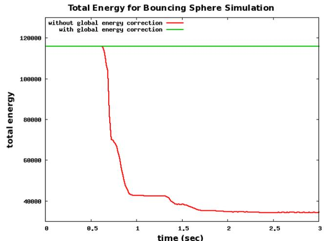
Fig. 14. A graph showing the total energy over time in the simulation of the coarse tetrahedralized sphere shown in Figure 2. The red line is the total energy when our energy conservation scheme is not used, whereas the green line is the total energy when utilizing our new scheme. The sudden declines in the red line correspond to collisions between the sphere and the ground.
