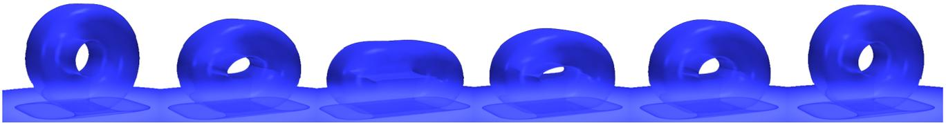
Fig. 15. A deformable wheel is dropped from a height and collides with the ground and itself, producing both rigid/deformable and self-collisions. Our global energy correction technique is used to restore all energy lost during evolution and collisions, allowing the wheel to bounce to its original height.
