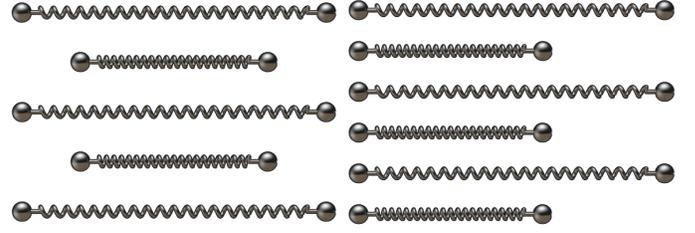
Fig. 3. (Left) A single unconstrained spring released from a stretched state and evolved using our new spring force, allowing it to continue to oscillate about the restlength. (Right) A single spring constrained at the left endpoint, released from a stretched state and evolved using our new spring force, allowing it to continue to oscillate about the restlength. Note that we chose a time step equal to the size of the framerate for both simulations.
