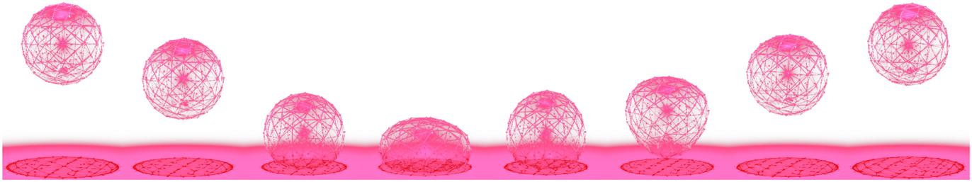
Fig. 2. Our global energy correction technique is used to restore all energy lost during evolution and collisions, allowing the sphere to bounce to its original height. It also restores energy lost from damping, as this simulation uses the semi-implicit Newmark scheme from [8].
