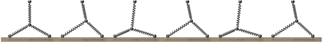
Fig. 7. Three springs constrained at their non-shared endpoints, where the shared node is given an initial velocity to the upper right. The shared node is then released and the springs are evolved using our new spring force, allowing the shared node to continue to oscillate back and forth. The time step size is set equal to the framerate of the simulation.
