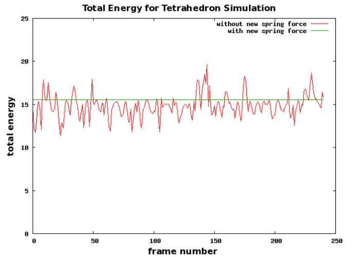
Fig. 9. A graph showing the total energy at the end of each frame in the simulation of a single tetrahedron with altitude springs shown in Figure 8. The green line shows the energy using our new energy conserving spring forces, and the red line shows the total energy if normal spring forces were used for that frame.
