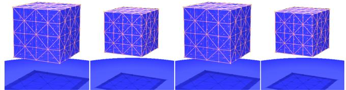
Fig. 1. Our global energy correction allows one to use damping to improve the aesthetics of a simulation while maintaining energy conservation, enabling a stretched cube to oscillate uniformly in and out while exactly conserving energy. In contrast, the variational integrator seen in [14] exhibits either high speed oscillations when exactly conserving energy or loss of energy when damping is added to make the simulation more visually appealing.
