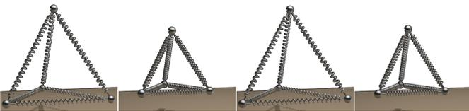
Fig. 8. A single tetrahedron with edge and altitude springs is stretched and then released. It is evolved using our new spring force, which allows it to oscillate back and forth continuously about its rest state. The time step size of this simulation is set equal to the framerate.
