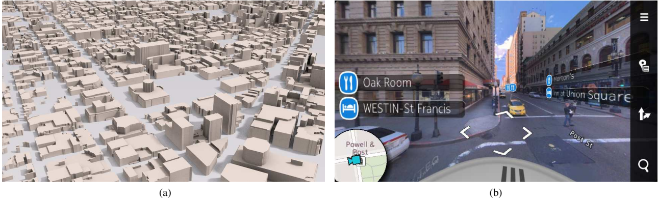
Figure 1: (a) A 3D city model automatically created using the proposed method. (b) A screenshot from Nokia City Scene, a mobile augmented reality application that uses the 3D city model to create a natural-looking augmentation of an urban scene.
