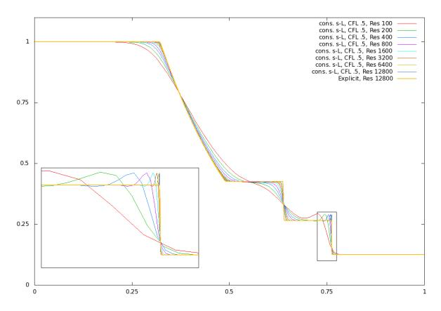
Figure 20: Density profile of a SOD shock tube at t = .15s, as generated by the scheme detailed in [21], using our new conservative semi-Lagrangian scheme and a CFL number of .5. We zoom in to the box  $[.725, .775] \times [.1, .3]$ , showing the shock front in greater detail and highlighting convergence at the discontinuity.
