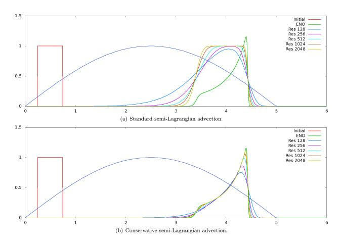
Figure 7: A square wave that evolves with a divergent velocity field  $u = \sin(\pi \frac{x}{5})$ . Shown is the solution at time t = 3s. We apply the first order version of both the standard semi-Lagrangian advection, as well as our proposed conservative semi-Lagrangian advection scheme. In this example, we see the standard semi-Lagrangian advection scheme converges to the wrong solution.
