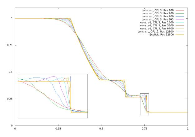
Figure 21: Density profile of a SOD shock tube at t = .15s, as generated by the scheme detailed in [21], using our new conservative semi-Lagrangian scheme and a CFL number of 3. We zoom in to the box  $[.725, .775] \times [.1, .3]$ , showing the shock front in greater detail and highlighting convergence at the discontinuity.
