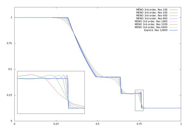
Figure 22: Density profile of a SOD shock tube at t = .15s, as generated by the scheme detailed in [21], using a third order MENO advection scheme and a CFL number of .5. We zoom in to the box  $[.725, .775] \times [.1, .3]$ , showing the shock front in greater detail and highlighting convergence at the discontinuity.
