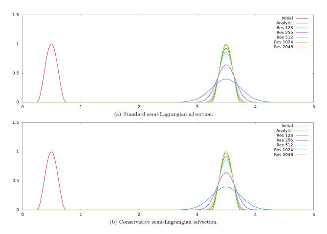
Figure 2: A sine-wave "bump" is advected through a uniform velocity field. Shown is the solution at time t = 3s. We apply the first order version of both the standard semi-Lagrangian advection, as well we our proposed conservative semi-Lagrangian advection scheme.
