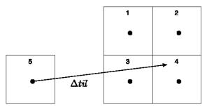
(b) Cell 5 casts a ray forward,  $\Delta t \vec{u}$ , which lands between cells 1, 2, 3 and 4. We again use standard bilinear interpolation, giving forward-cast weights  $f_{51} = .06$ ,  $f_{52} = .24$ ,  $f_{53} = .14$ ,  $f_{54} = .56$ .
