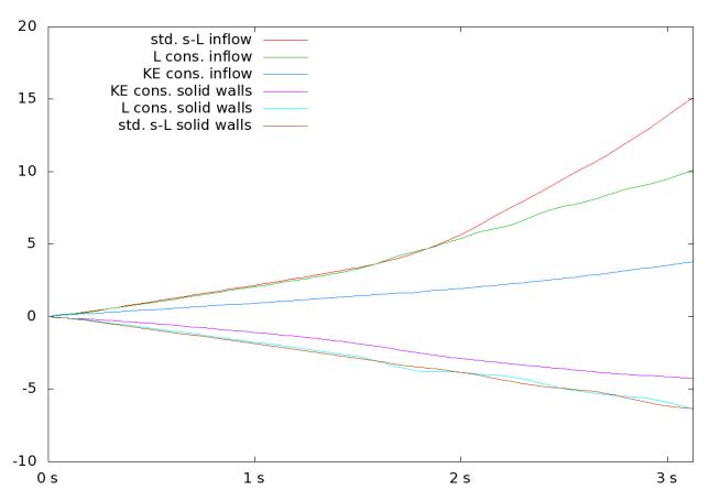
Figure 14: Pressure momentum flux into solid wall boundaries, and pressure momentum flux entering the computational domain from the inflow boundary condition, plotted as a function of time for a standard semi-Lagrangian scheme and our proposed momentum-conserving scheme.
