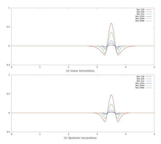
Figure 3: Error curve for the advected sine-wave "bump" in a constant velocity field u = 1 at time t = 3s for linear and quadratic interpolation using our proposed conservative semi-Lagrangian advection scheme, run with a CFL number .9. Using a higher-order interpolation scheme gives noticeably reduced error; for example at  $\Delta x = 5/256$  the peak error for the linear interpolation scheme is .111, while the quadratic interpolation scheme has a peak error of .060.
