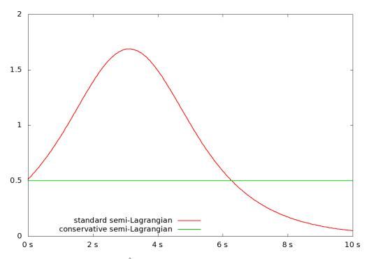
Figure 8: Shown is the time history of  $\sum_i \Delta x \hat{\phi}_i$  for a square wave that is evolved through a divergent velocity field with  $u = \sin(\pi \frac{x}{5})$ . Solutions for both the standard semi-Lagrangian advection scheme and our proposed conservative semi-Lagrangian advection scheme are shown at high-resolution with  $\Delta x = 5/8192$ .
