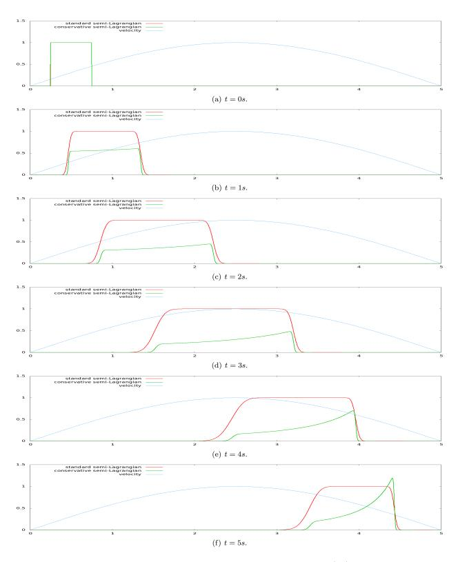
Figure 6: We consider the evolution of density in a velocity field that is specified by  $u(x) = \sin(\pi \frac{x}{5})$ . In such a velocity field, the standard semi-Lagrangian approach fails to capture the rarefaction and converges to a non-physical solution. This simulation is run with  $\Delta x = 5/8192$ .
