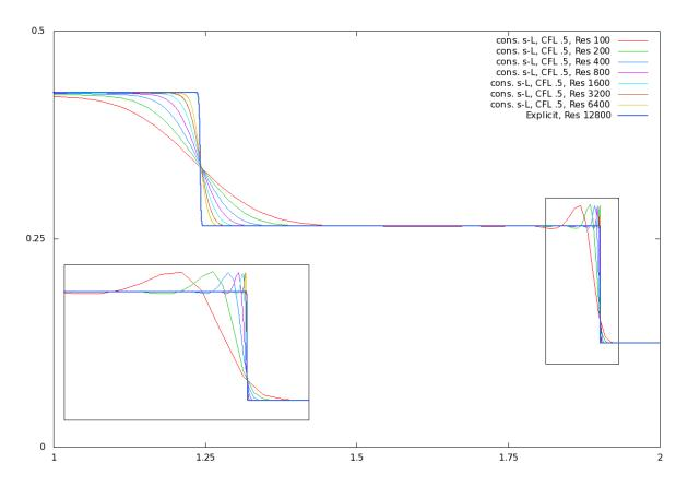
Figure 23: Density profile of a SOD shock tube at t = .8s, as generated by the scheme detailed in [21], using our new conservative semi-Lagrangian scheme and a CFL number of .5. In order to capture this later time, we extend the computational domain to  $x \in (-1, 2)$  and show only  $x \in (1, 2)$  to illustrate shock front convergence. We zoom in to the box  $[1.812, 1.932] \times [.1, .3]$ , showing the shock front in greater detail and highlighting convergence at the discontinuity.
