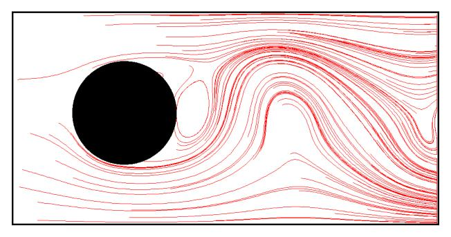
Figure 12: Stream-line visualization of flow past a sphere.
