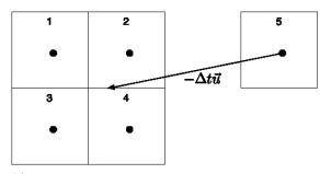
(a) Cell 5 casts a ray backward,  $-\Delta t \vec{u}$ , which lands between cells 1, 2, 3 and 4. Using a standard bilinear interpolation scheme, the weights are calculated to be  $w_{15} = .125, w_{25} = .375, w_{35} = .125, w_{45} = .375.$
