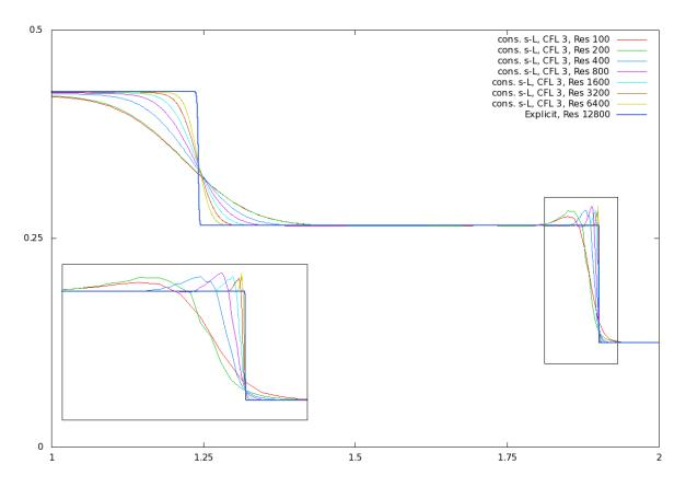
Figure 24: Density profile of a SOD shock tube at t = .8s, as generated by the scheme detailed in [21], using our new conservative semi-Lagrangian scheme and a CFL number of 3. In order to capture this later time, we extend the computational domain to  $x \in (-1, 2)$  and show only  $x \in (1, 2)$  to illustrate shock front convergence. We zoom in to the box  $[1.812, .932] \times [.1, .3]$ , showing the shock front in greater detail and highlighting convergence at the discontinuity.
