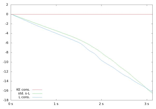
Figure 19: Sum total of kinetic energy in the domain, plus kinetic energy fluxed out of the domain (through outflow and solid wall boundaries), minus kinetic energy fluxed into the domain (through inflow), plus kinetic energy lost in the projection step away from boundaries, plotted as a function of time for a standard semi-Lagrangian scheme, our proposed momentum-conserving scheme, and our proposed kinetic energy-conserving scheme.
