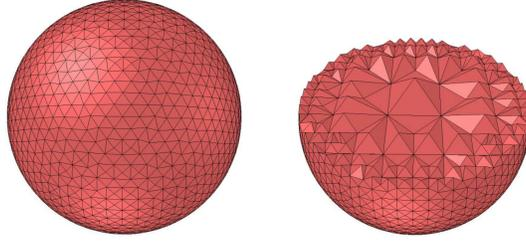
**Figure 3: Tetrahedral mesh of a sphere (18K elements). The cutaway view illustrates that the interior mesh can be fairly coarse even if high resolution is desired on the exterior boundary.**
