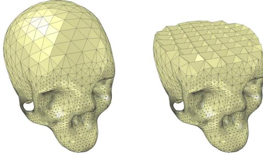
**Figure 6: Tetrahedral mesh (left) and cutaway view (right) of a cranium (80K elements).**
