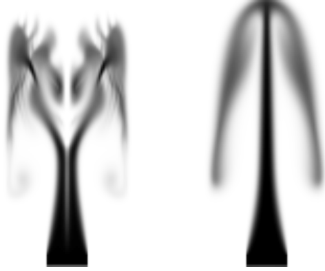
Figure 2: (Left) using the method from [LGF11], incompressibility is not properly enforced on coarse grids with large time steps and no viscosity. Note the white line down the middle of the image where the smoke splits apart, which occurs because of a lack of incompressibility during the advection. (Right) our new method incorporates incompressibility into advection, keeping the plume from splitting apart.
