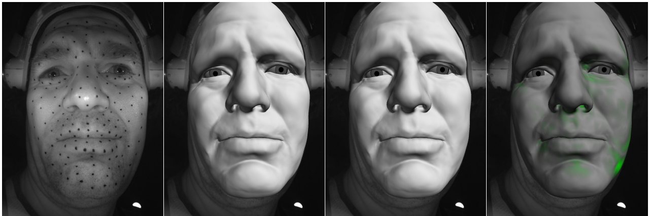
Fig. 7. Far Left: Helmet mounted camera footage. Middle Left: The reconstruction obtained using our approach captures a subtle expression in the helmet mounted camera footage. This performance also shows the effectiveness of our temporal smoothness constraints. See video in supplementary material. Middle Right: Adding simulated in-betweens allows us to improve the smoothness of the reconstruction in the philtrum and the right jowl while also improving the lift in the upper right cheek. Far Right: Heatmap highlighting the differences between (Middle Left) and (Middle Right).
